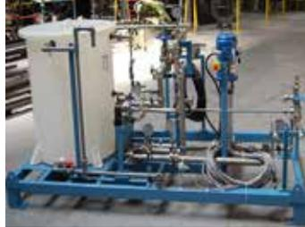
Mounted on a support structure, this skid is used to cool down the plasma torch with de-ionized water in a closed loop circuit.
