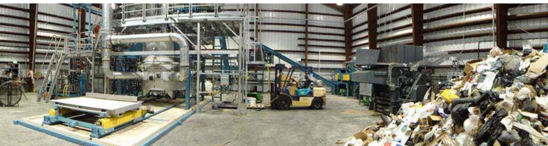
Since the PRRS is a much more compact unit as compared to traditional waste treatment or disposal, the process offers outstanding versatility. The syngas produced by the PRRS can be used to produce electricity to power the system, steam or even biofuels. The air emissions from the PRRS complies with all current regulations, offering an environmentally friendly solution to landfill and incineration while also producing energy and construction materials.
